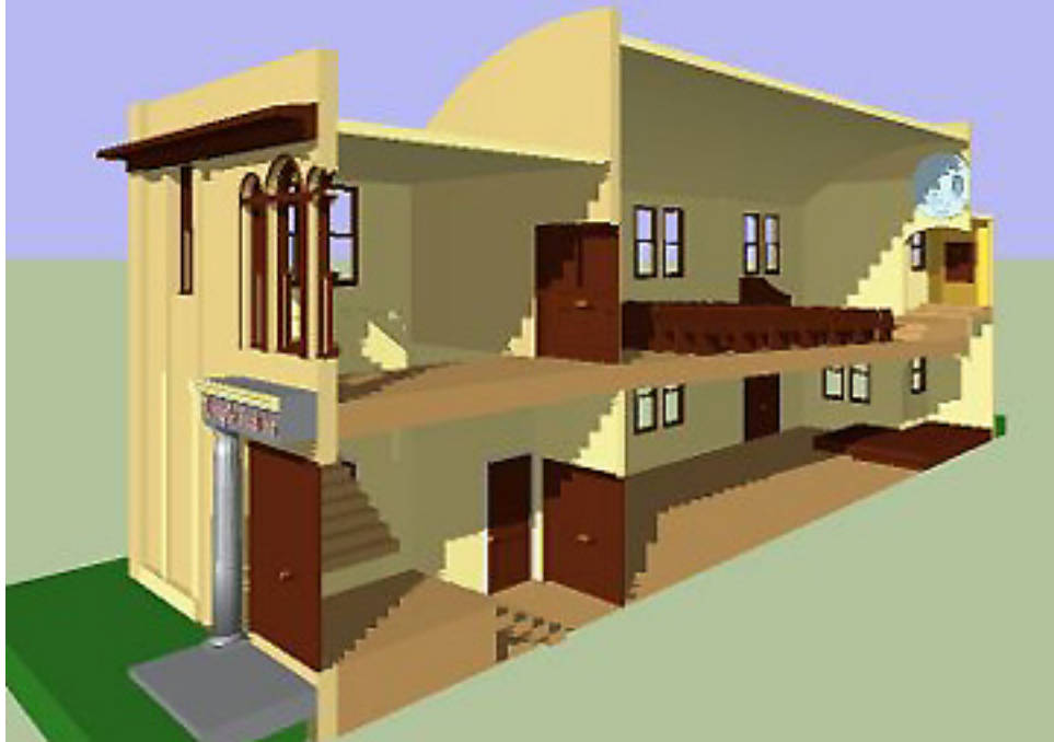
The double-decker assembly halls served a congregation which was, at least in the early years, both Reform and Orthodox requiring simultaneous but separate facilities. The raked (sloped) upper floor is characteristic of the audience/presentation aspect of Reform, while the flat floor below better served the participatory service-in-the-round aspect of the typical Orthodox minyan.
