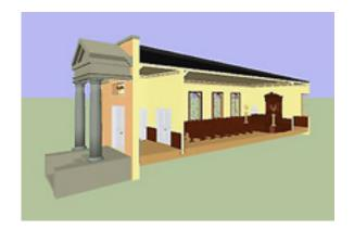
The interior plan consists of a foyer with flanking wc and service rooms, the main sanctuary, and meeting room in the rear. Despite its small size  $(60' \times 25' \text{ overall})$  the floor is raked, effectively (and conceptually) separating the congregation from the activity on the pulpit as it would be in a theater. Contrast this style of worship with the Orthodox Shule in Brenham with its central bimah where the congregants would have actively participated in and led the services.
