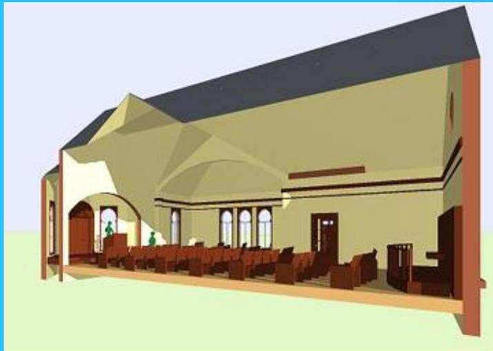
The sectional view is from the opposite direction of the birdseye view above. The ark stands in an apse on the east, opposite the choir loft and Tracker organ (pipes omitted to show rose window) on the west. In the original the plaster corners at the intersections of the roof planes were rounded to give the impression of arched vaults.
